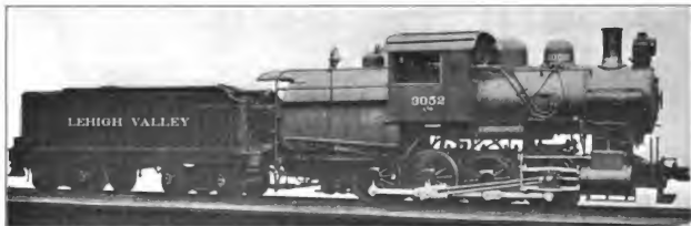
Fig. 19. Eight-Wheel (0-8-0) Switching Locomotive. Built by the Baldwin Locomotive Works for the Lehigh Valley. Cylinders 21 in. x 28 in., Working Steam Pressure 200 lbs. per sq. in., Heating Surface 2,248 sq. ft., Diameter of Drivers 55½ in., Weight on Drivers 172,450 lbs., Total Weight 172,450 lbs.
